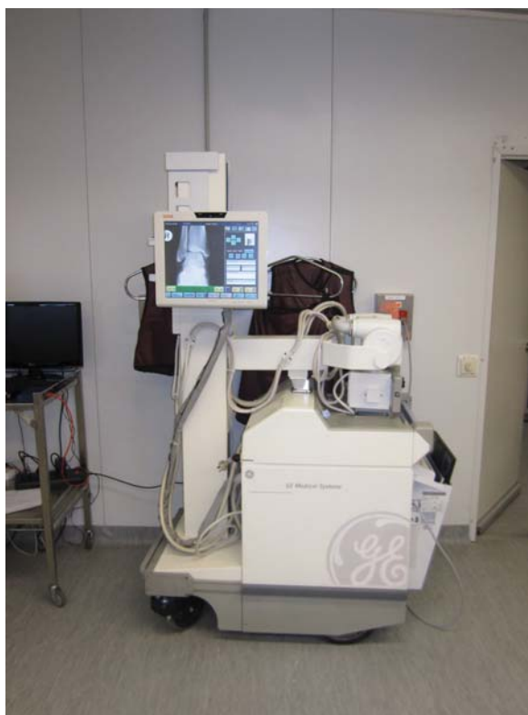
State-of-the-art digital radiography unit with wireless detector from Carestream, which is attached to an AMX 4 plus portable x-ray unit at the trackside medical facility
